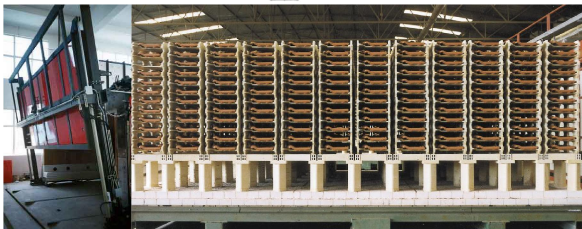
A typical layout of the shuttle kiln along with kiln cars and transfer handling system
